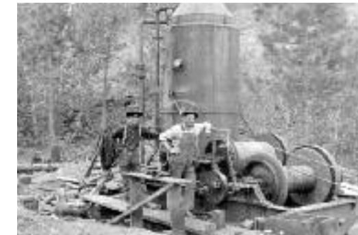
Donkey engines came in many different styles like this double-drum donkey. They could relocate under their own power by being tied to trees and winning themselves forward, even though they weighed about 10 tons. It must have been something to see them in operation....rumbling, belching monsters in the woods!
